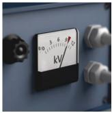
Testing the tool for dielectric strength at 10,000 volt gives the user the peace of mind that their tool has been tested for its most important property, insulation. Wera VDE tools are subjected to this test piece by piece which guarantees safe working at up to 1,000 volt.
